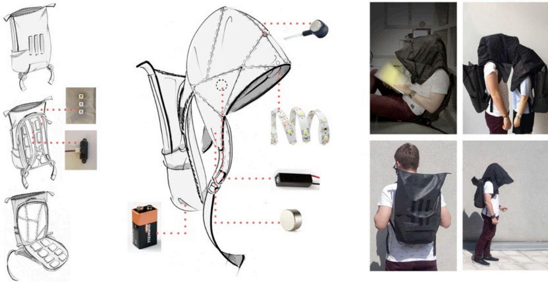
Fig. 2: Hut Hood. It is a convertible backpack with an integrated hood that doubles as a portable study: it creates a private space that affords the wearer concentration whenever required and under all circumstances. The hood shuts out the environment and selectively obliterates or amplifies environmental sounds, while the backpack can be turned into a comfortable seat on which to work.
