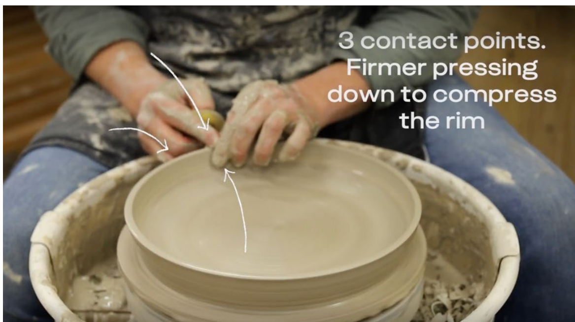
Fig 6. Decoding Ceramics (no date) Augmenting video demonstration to reveal hidden embodied expertise.
