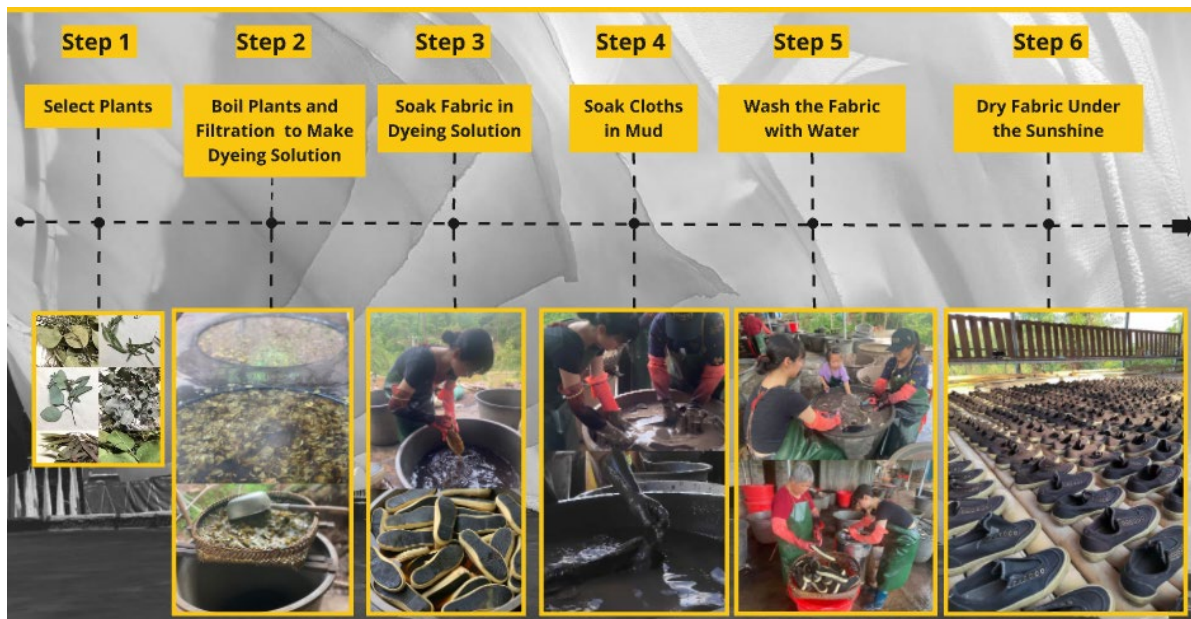
Fig 3. Yan Feng (no date) Mud-dyeing Process Flowchart
