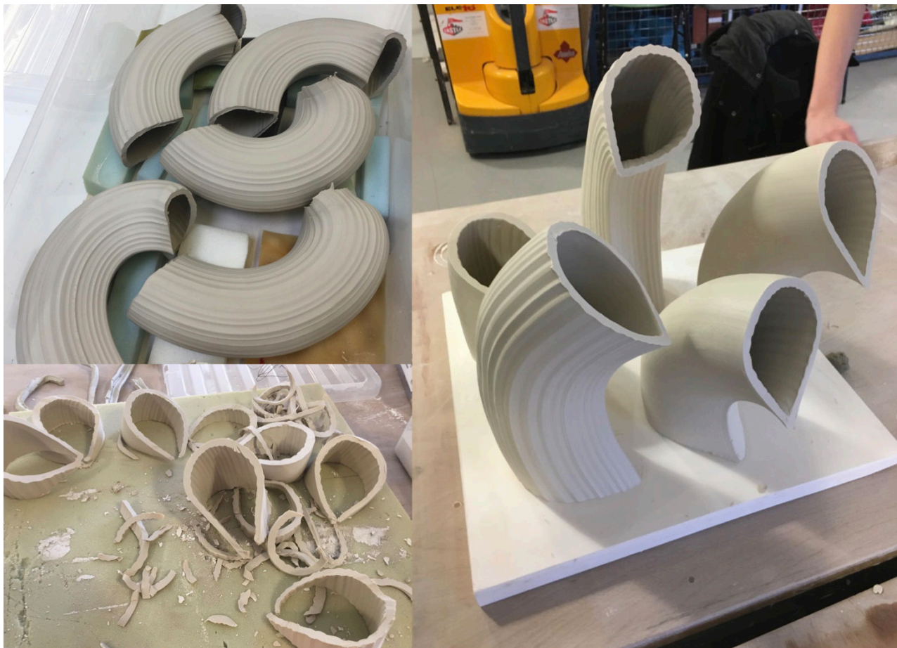
Fig 5: Images illustrating part of the workflow for creating the Jugs. Extruded shapes resting on foam pieces to harden (top left image), scraps from the trimming process is illustrated in bottom left image, and jugs placed on plaster bats to form the bases is illustrated on the image to the right. Photos: T. Jorgensen, 2016.
