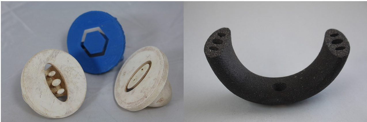
Fig 1: 3D Printed Extrusion Dies by Taslim Martin, with extruded clay form on the right. Images: T. Martin 2016
