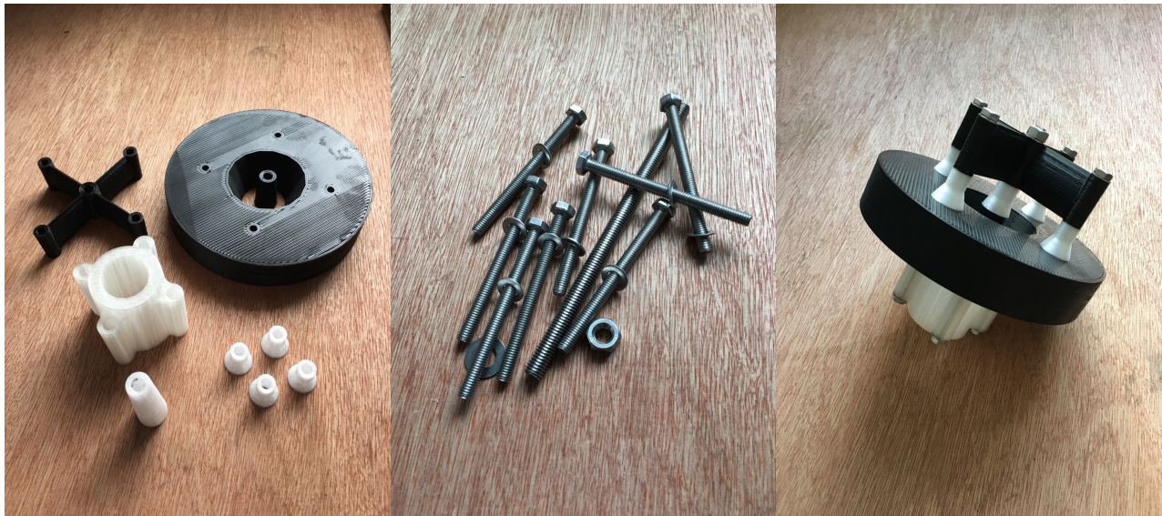
Fig 12: Components for a 3D printed dies, with the printed components to the left, stainless steel bolts centre and the complete assembled extrusion die on the right. Photos: T. Jorgensen, 2020.
