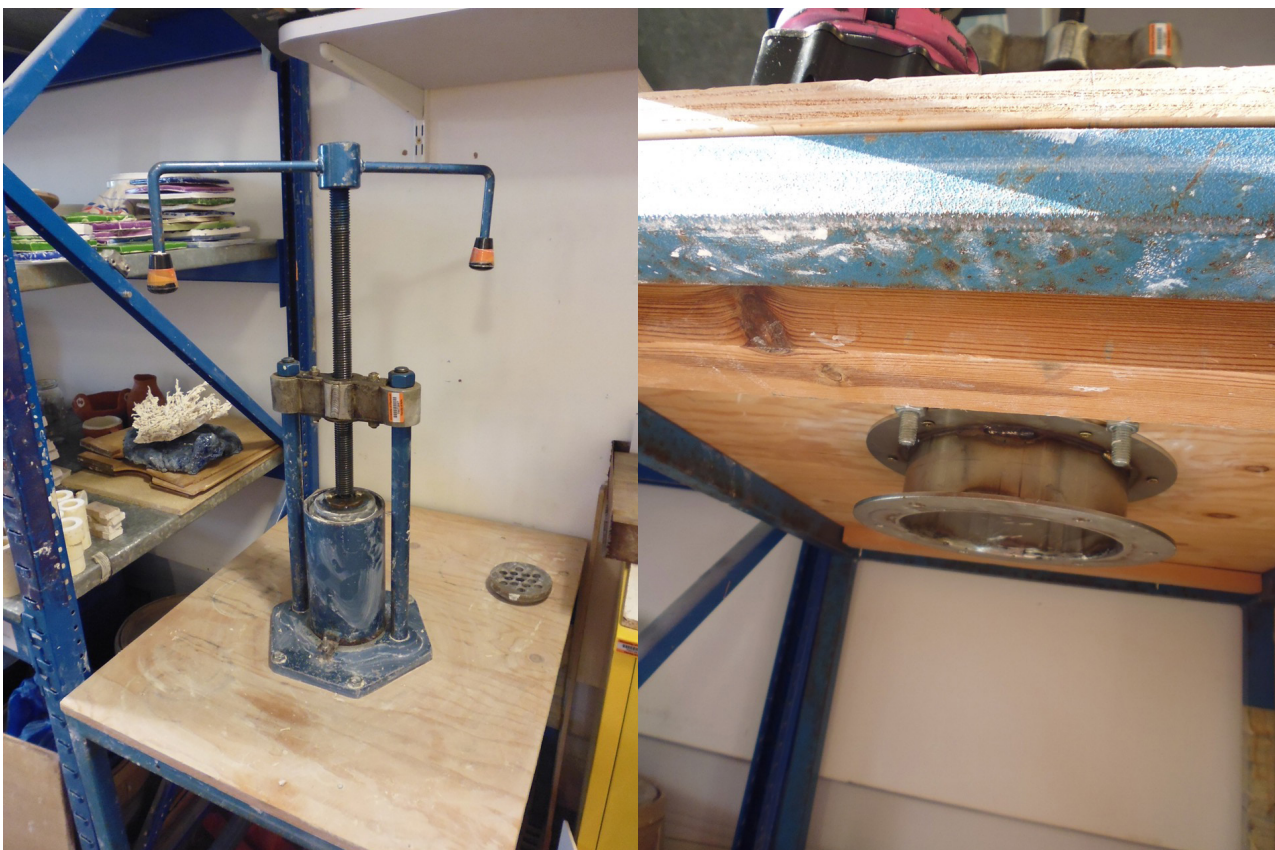
Fig 2: Screw action piston extruder used for the initial tests undertaken by the author, the expansion box that facilitates larger diameter die is illustrated in the image to the right. Photos: T. Jorgensen, 2016.
