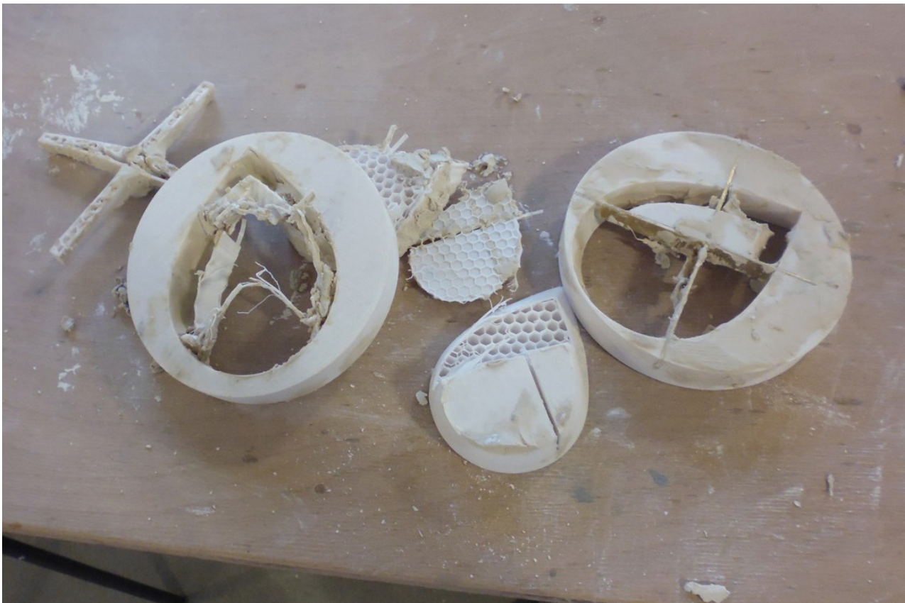
Fig 3: Failed 3D printed dies due to the extrusion pressure, with the characteristic sparse interior infill revealed. Photo: T. Jorgensen, 2016.
