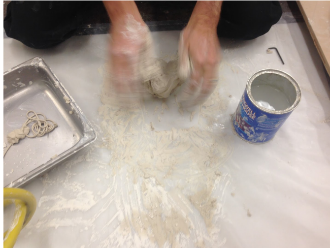
Figure 2: Mixing clay prior to printing
