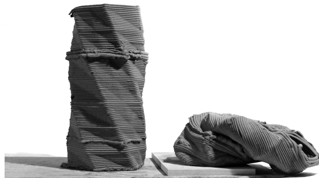
Figure 3: Printing to failure
