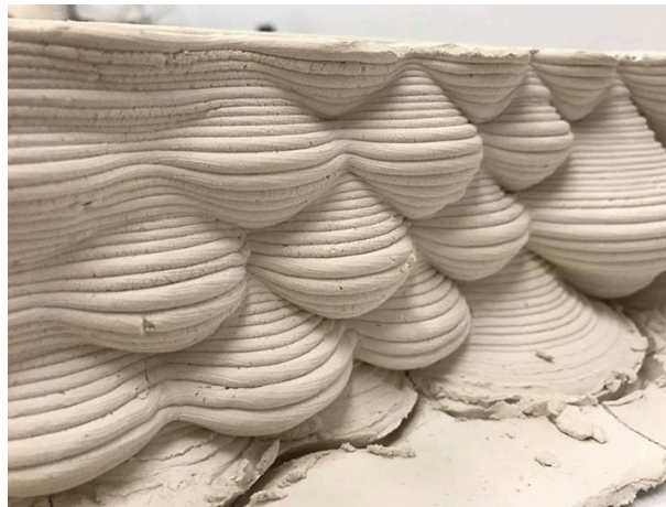
Figure 2: Early attempts at hand control of clay flow rate
