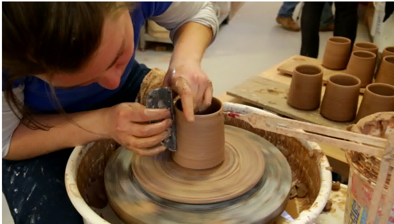
Figure 1. Kat Wheeler ribbing a Leach standard ware mug cylinder using a D-shaped wooden rib tool (type A ribbing). Image: Salani, 2016.
