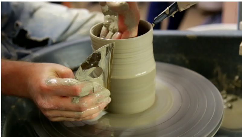
Figure 2. Florian Gadsby ribbing a Maze Hill mug with a metal rib, from the bottom up (type B ribbing). Image: Salani, 2016.
