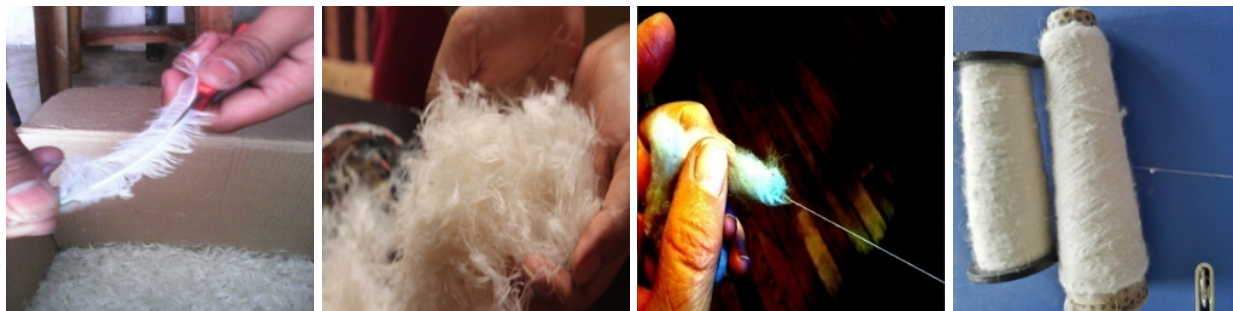
Fig.1.13 Separating chicken feather fibres, Fig.1.14 Fibre blending, Fig.1.15 Hand spinning, Fig.1.16 Yarn
