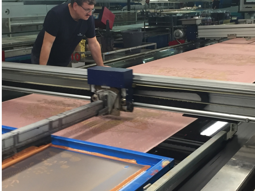
Figure 3: A Screen printing expert oversees traditional mechanised textile print production at Mantero.
