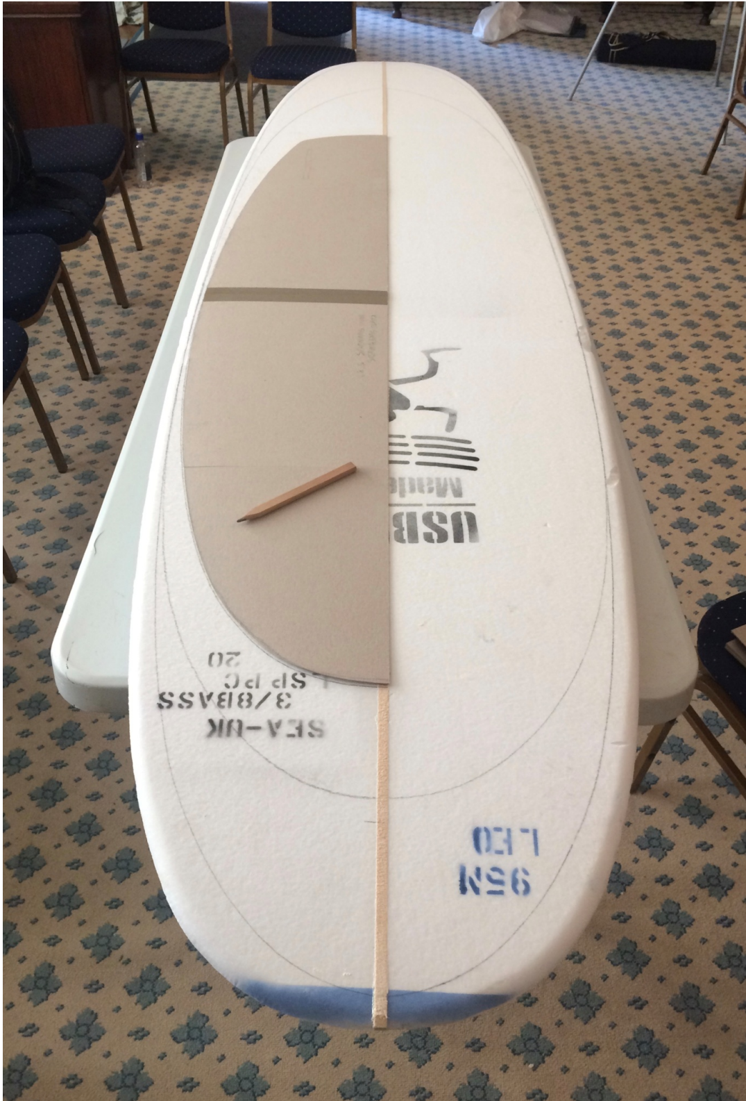
Prototype for user remanufacture: a polyurethane surfboard blank marked out with three concentric templates for beginner-intermediate use. Image: Paul Kerlaff / Making Futures 2017)
