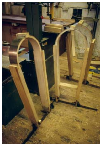
Fig 6. C3 main bends still in compression straps (Photo Trannon)
