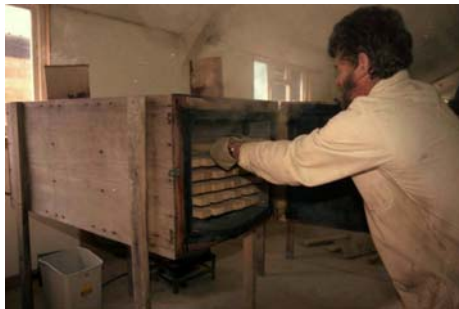
Fig 4. Removing pairs of blanks from steam box after 1 hour (Photo Trannon)
