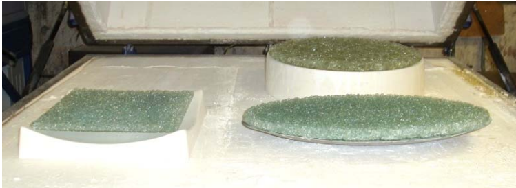
Figure 12, Production of bowls and plates for the show apartment before slump
