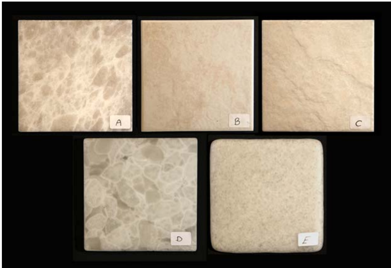
Figure 16, Tiles to be tested: A=stone, B=c.thin, C=c.thick, D= l.g.d.glass and E=gwalia
