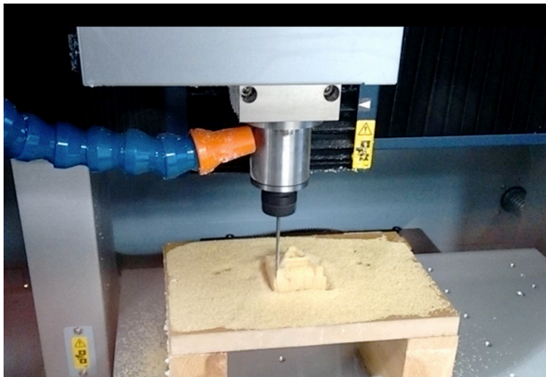
Figure 4 : Gill Sans capital 'a' prototype, cut using digital milling machine at Plymouth College of Art Fab
