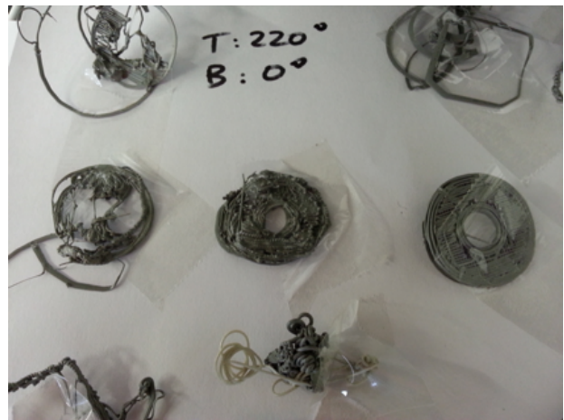
©Co-product CIC. Range of failed print tests.
