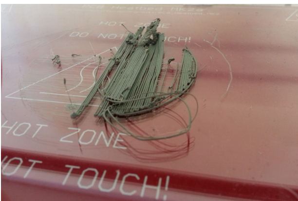
©Co-product CIC. Failed print job, due to inconsistent filament.
