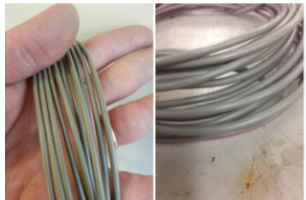
©Co-oproduct CIC. Examples of successful production of consistent filament from waste PP
