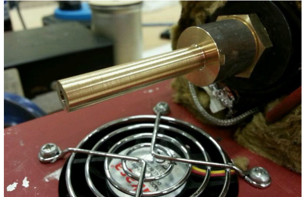
©Jamie billing. New filament extruder nozzle produced at NTU by Kerry Truman.
