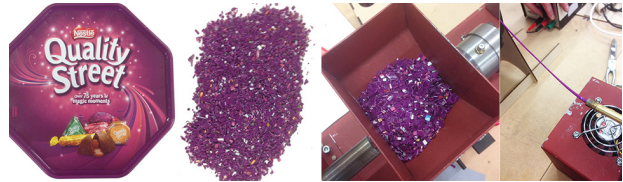
©Co-product CIC. Quality Street shredded & extruded into printable filament.
