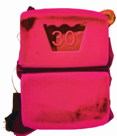
Fig. 4. Polyester clothing moulded into a two sided rigid shell for a clasp bag.
