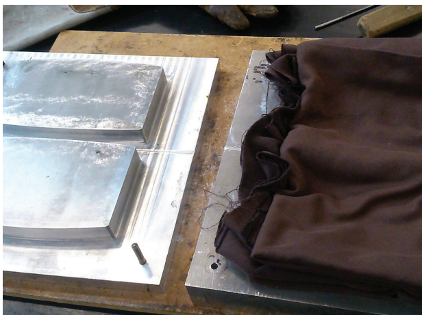
Fig. 2. Layering of materials in an aluminium compression mould.
