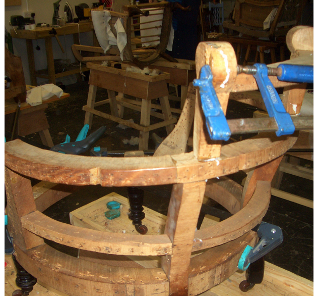
Figure 7: The repairs necessary to ensure a safe and sturdy chair frame are shown in the image. The clamps hold the frame in place while the wood glue dries around the wooden dowels.
