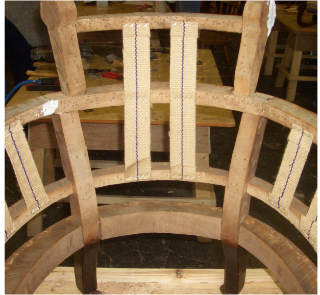
Figure 2: The stripped chair frame with new webbing.
