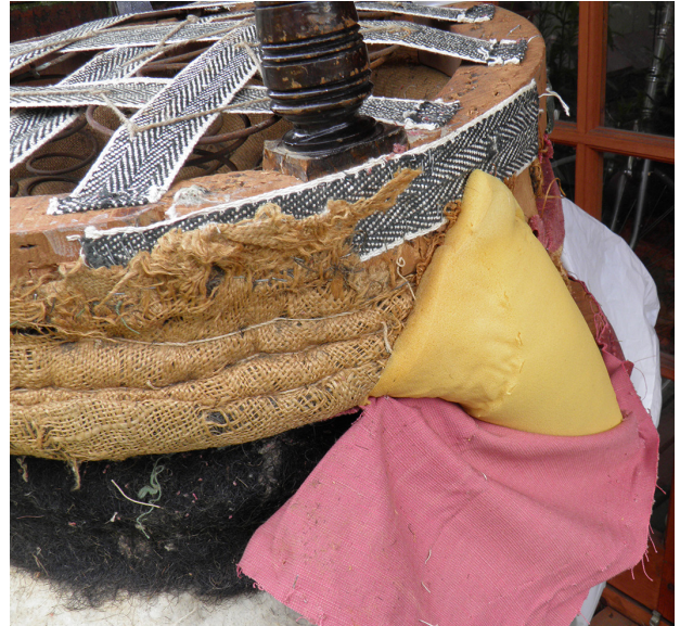
Figure 6: image shows the original stuffing materials that were exposed when removing the top fabric and the foam stuffing that had been applied during the previous re-upholstery work.
