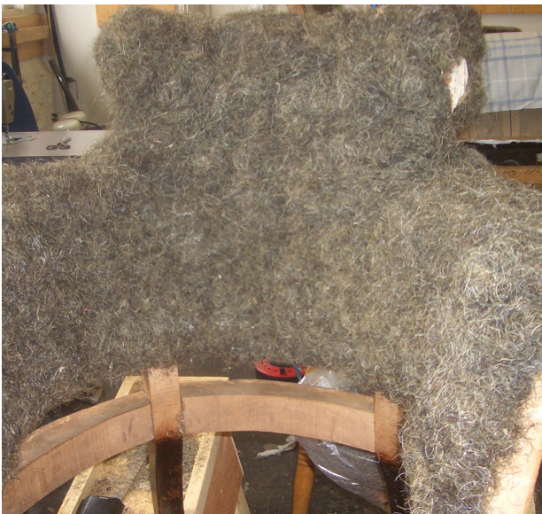
Figure 3: The chair frame with the beginnings of the horse hair stuffing applied to the inner back and sides (traditional materials and techniques).
