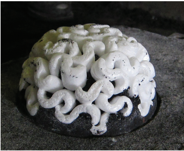
Fig. 6 Polystyrene pellets, glued together, are immersed in the sand to make a waste mould.
