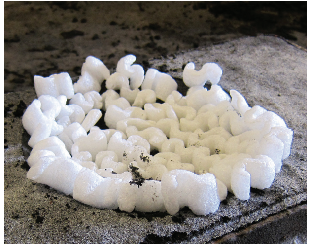
Fig. 4 Polystyrene packaging pellets as a waste mould. (Lambert 2015)
