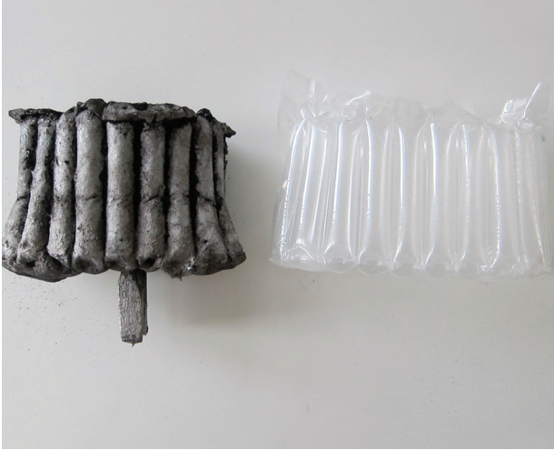
Fig. 14. Sandcasting of airbag packaging. (Lambert 2015)
