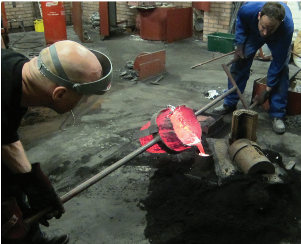
Fig. 10 Pouring molten aluminium into sandcasts
