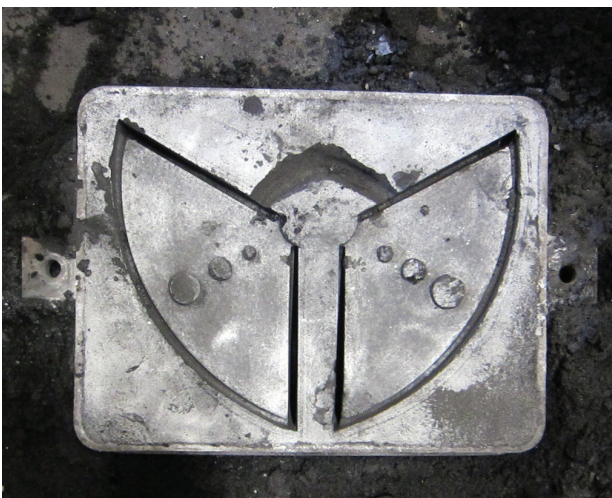
Fig. 3. Sandcasting mould using MDF patterns in a two part mould to create a cavity. (Lambert 2014)
