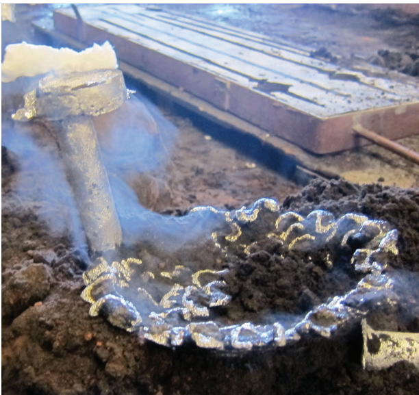
Fig 2 Resulting casts with the sprue still attached.
