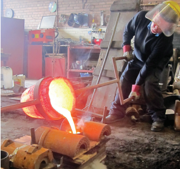
Fig.1 Pouring molten aluminium into sandcasts; (Author, 2015)
