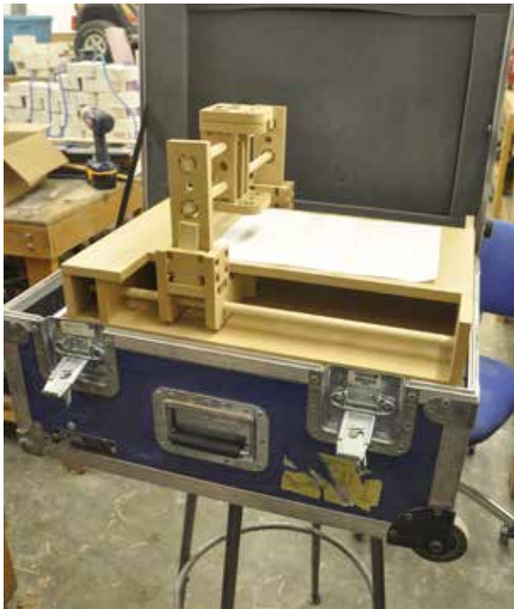
Figure 4. Wood prototype – Suitcase CNC.
