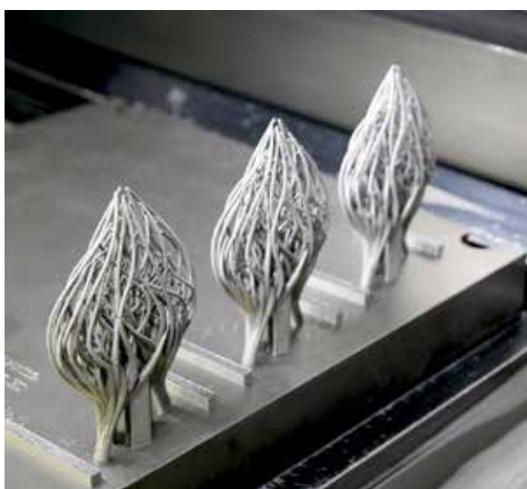
Figure 12: Cuore pendants on the build substrate. Photograph: John Vickers 3T RPD Ltd
