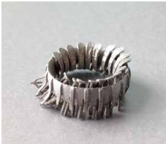
Figure 15: First test with deformed radial arrays after removal from the base plate.
