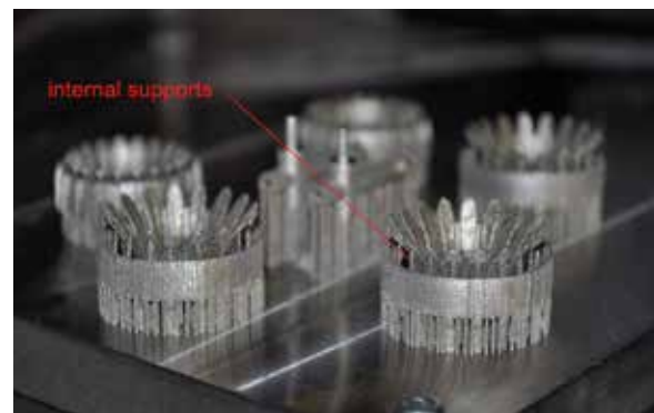
Figure 16: Test pieces on base plate with additional internal supports, 2013.
