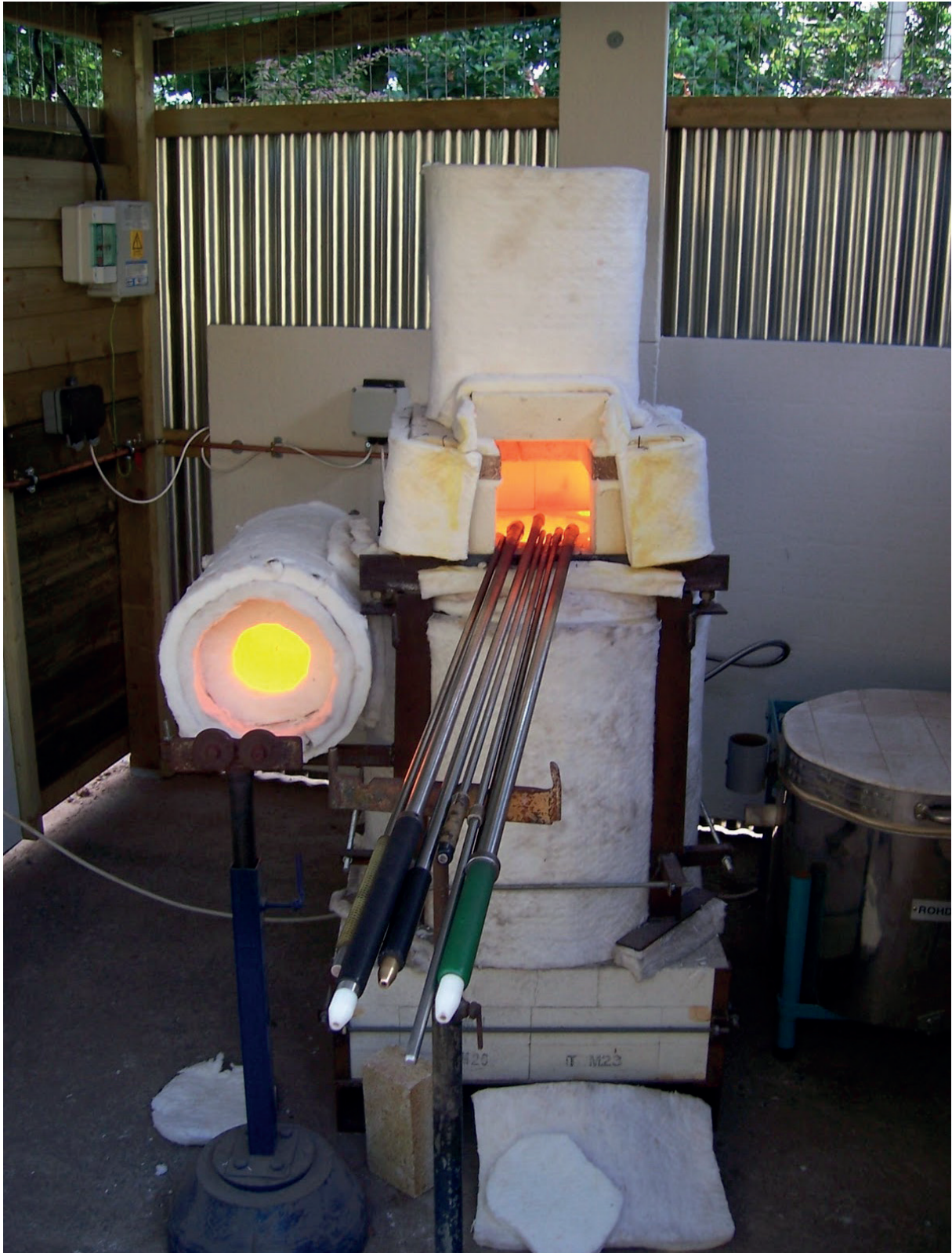
The RGH1 glass furnace, developed on 17 th century thinking with cutting-edge materials and computer-controlled high/low combustion system. It cuts down the cost of running a professional studio by 75% running on natural gas, while enabling excellent glass quality.
