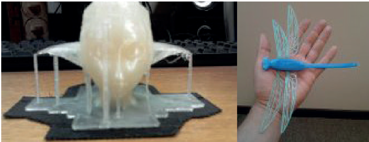
Top left – Pixie head, from a Maya animation file. The file caused glitches as it was imported into Axon 2 to enable it to be printed. I imported it into Rhino first, constructing a secondary raft and built support posts to hold the structure while being built. Note the messy result on the right ear, where the support fell away during the printing process.
