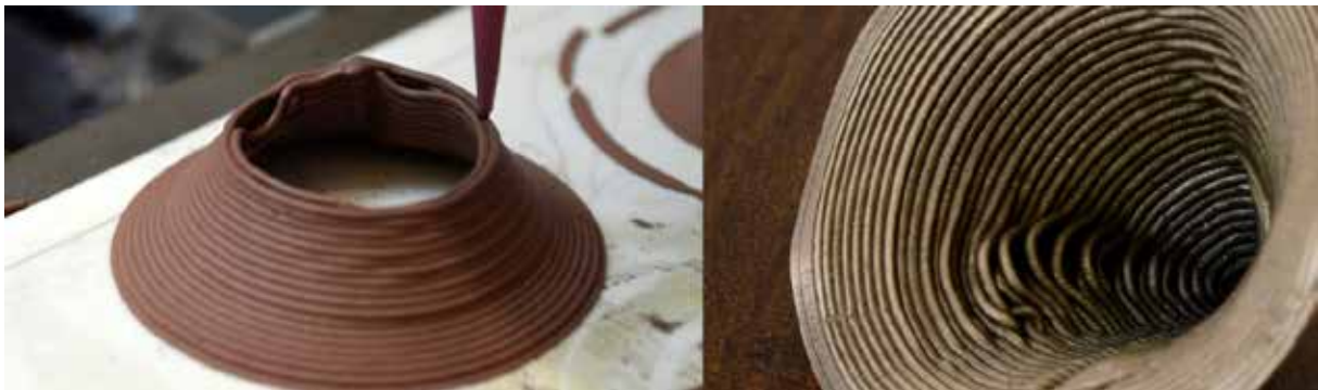
Figure 11. 40° draft angle cone, being deposited (left), fired (right), BronzClay. Esteban Schunemann (2012) © Esteban Schunemann.
