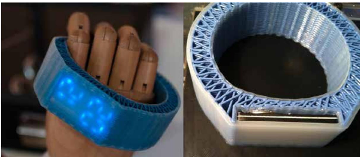
Figure 10. Silicone watch finished (left), movement installed (right). Esteban Schunemann (2012) © Esteban Schunemann.
