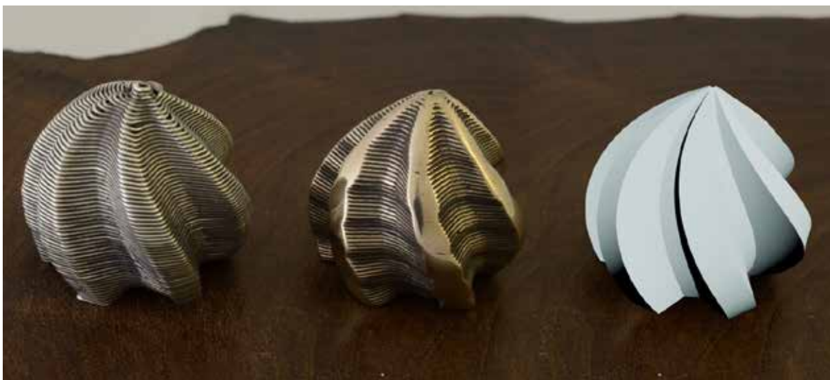
Figure 13. Seashell build in PMC Pro (left), BronzClay (middle) and CAD model (right). Esteban Schunemann (2012) © Esteban Schunemann.
