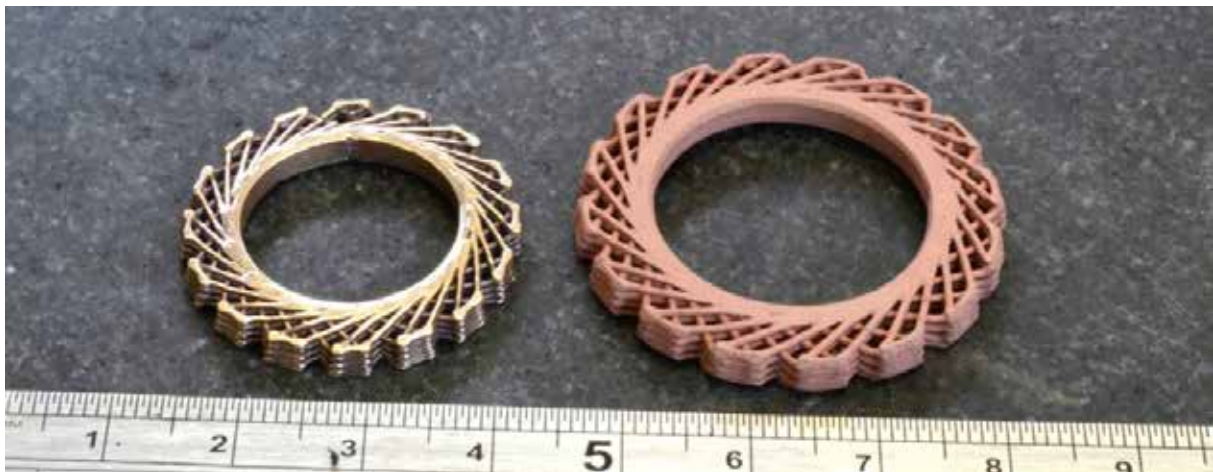
Figure 14. Tessellated ring shrinkage comparison in BronzClay. Esteban Schunemann (2012) © Esteban Schunemann.
