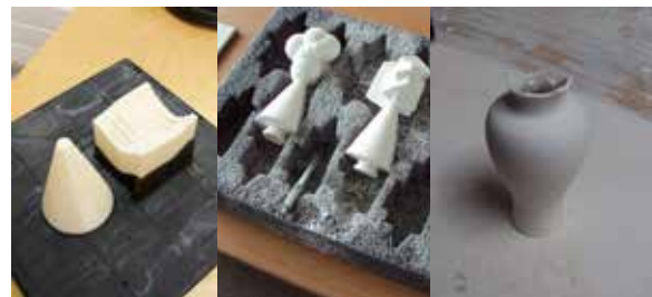
Figure 1. RP test models in ABS plastic and starch. RT mould printed in the zp150 material. Photo: Jorgensen 2010
